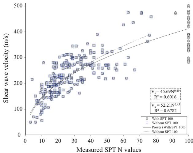
**Fig. 5** Combined shear velocity versus SPT N data and correlation excluding (dotted line and box) and including (solid line and box) N value of 100. Data from Bangalore, Chennai, Coimbatore and Vizag
