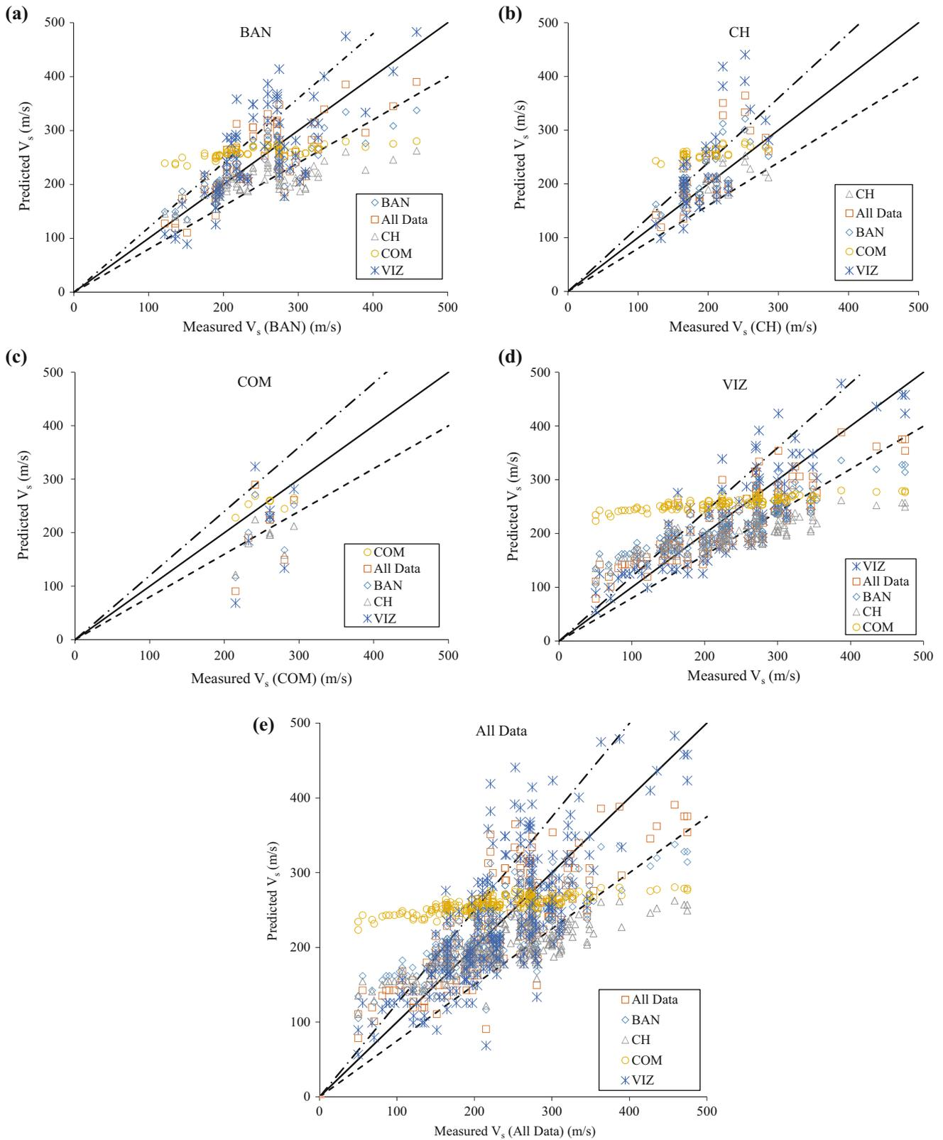
**Fig. 7** Comparison between measured and predicted  $V_s$  values for each city using different models given in Figs. 4 and 5 for four cities excluding SPT  $N$  value 100 **a** Bangalore (BAN), **b** Chennai (CH), **c** Coimbatore (COM), **d** Vizag (VIZ) and **e** all data
