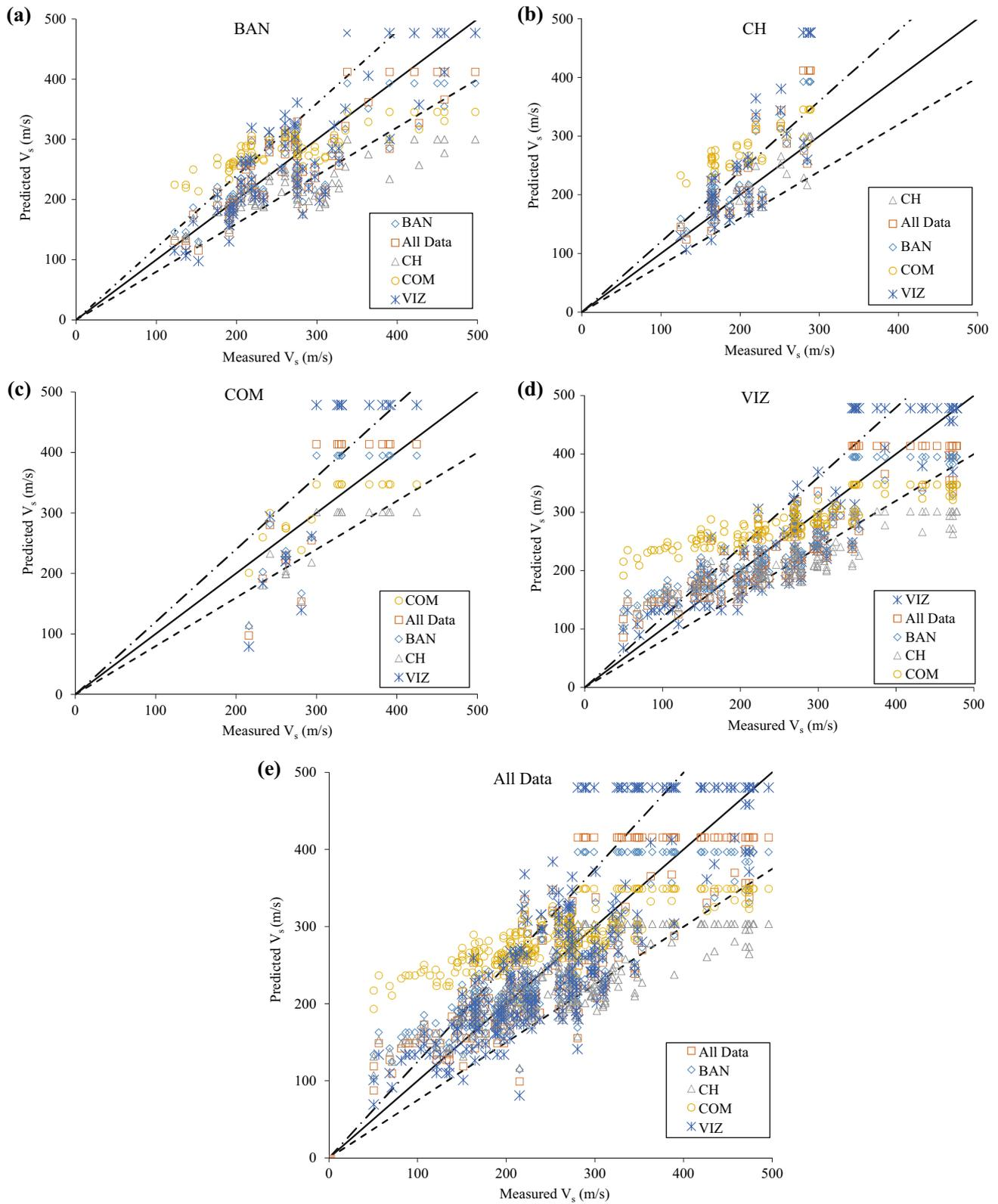
**Fig. 8** Comparison between measured and predicted  $V_s$  values for each city using different models given in Figs. 4 and 5 for four cities including SPT  $N$  value 100 **a** Bangalore (BAN), **b** Chennai (CH), **c** Coimbatore (COM), **d** Vizag (VIZ) and **e** all data
