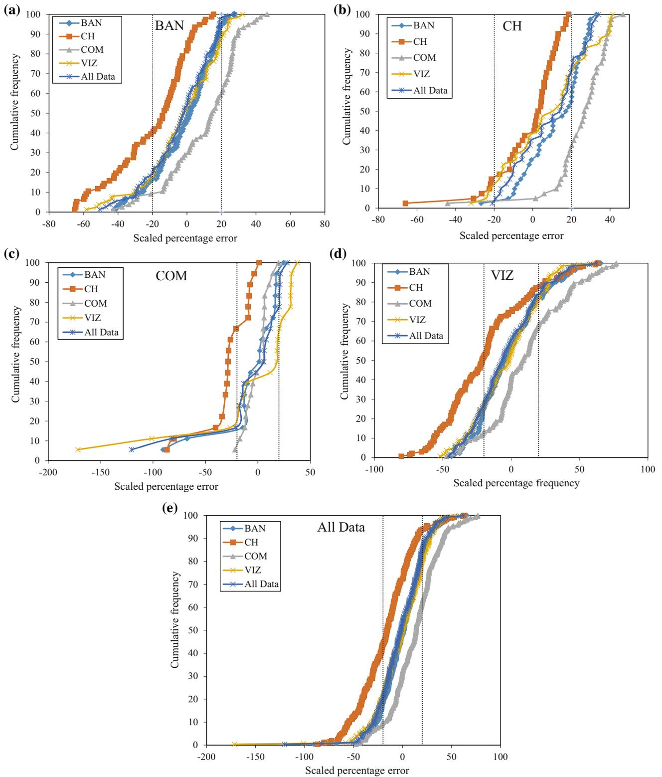
**Fig. 11** Scaled percent error for five correlations proposed for respective city and combined data. **a** Bangalore (BAN), **b** Chennai (CH), **c** Coimbatore (COM), **d** Vizag (VIZ) and **e** all data including SPT N 100
