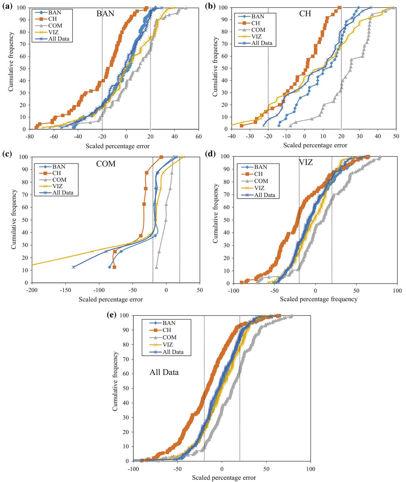
**Fig. 10** Scaled percent error for five correlations proposed for respective city and combined data. **a** Bangalore (BAN), **b** Chennai (CH), **c** Coimbatore (COM), **d** Vizag (VIZ) and **e** all data excluding SPT N 100
