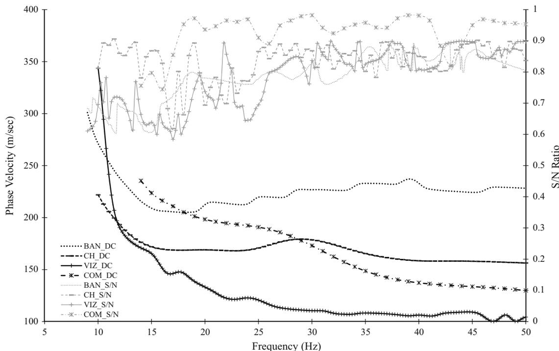
**Fig. 2** Typical dispersion curve (DC) and S/N ratio for Bangalore (BAN), Coimbatore (COM), Bangalore (BAN) and Vizag (VIZ)
