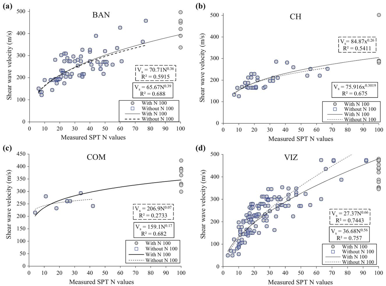
**Fig. 4** Shear velocity versus SPT-N data and correlation for four cities **a** Bangalore (BAN), **b** Chennai (CH), **c** Coimbatore (COM) and **d** Vizag (VIZ) with (solid line) or without (dotted line) including N
