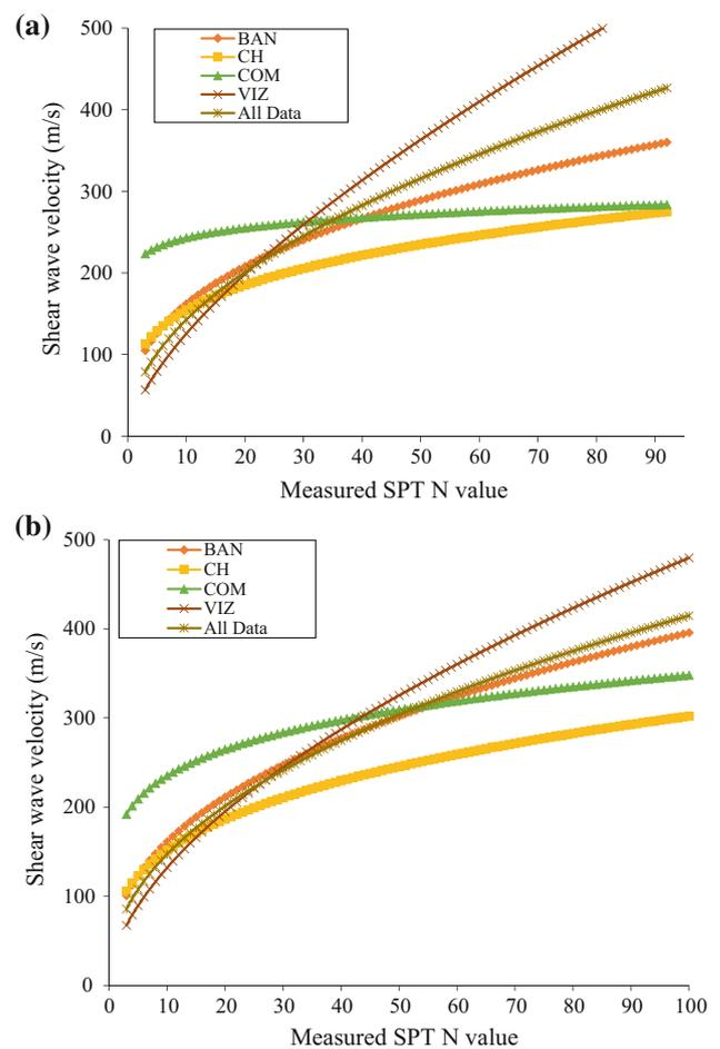
**Fig. 6** Comparison of shear wave velocity correlations developed in the study **a** excluding SPT N values 100 and **b** including SPT N values 100
